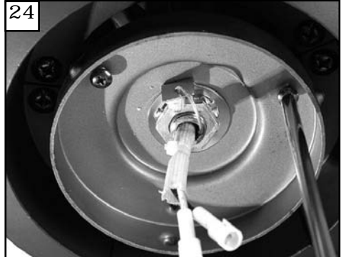
24 Loosen 2 screws and remove 1 screw to allow bottom fan plate to be installed.
